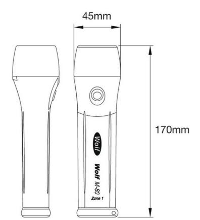
189 lumens LED Spot Beam (approx 7°) with a Wide Angle Fringe Beam (approx 55°)
