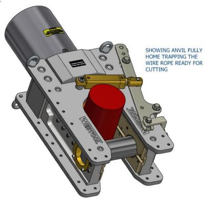
Operate the main ram down-stroke to sever the wire rope. Once the wire rope is severed, Pressurize the main ram retract port to withdraw the cutting blade. Then, and only then, retract the anvil. It is important not to operate the anvil cylinder whilst the main ram and blade are in the fully extended position.
