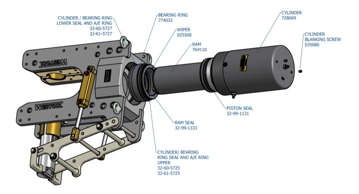
Put the assembled parts into a plastic dust bin or similar vessel, attach an oil supply to the coupling to the top of the cylinder, attach a hand pump to the coupling and pump out the ram, importantly, **by hand.**
