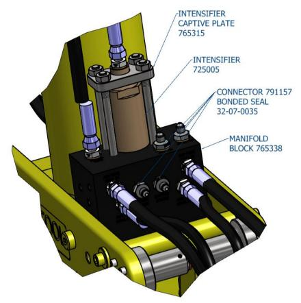
Below is shown a close up of the manifold block with hoses and connections removed for clarity, all hydraulic connection points are clearly marked, if any hoses are removed it is very important that they are replaced in the correct position.
