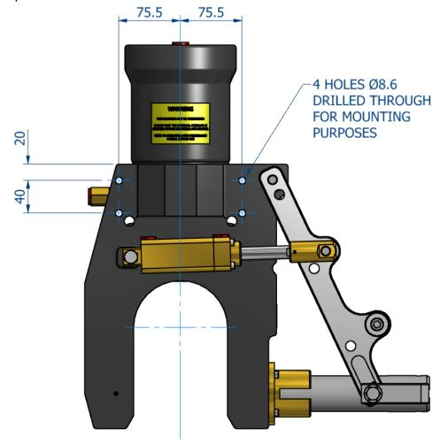
Two hydraulic supplies are required, one at 640 Bar, usually through an intensifier, for the main ram and another at 190 Bar max. for the auxiliary cylinders.
