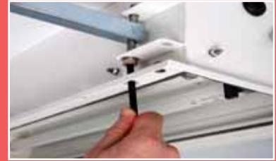
Single screw height adjustment
