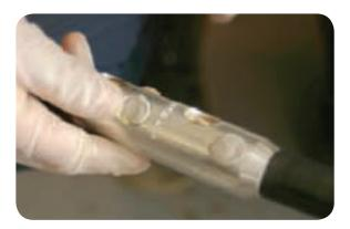
• Remove one of the backing sheets from the black mastic patch and position so that the connector is in the centre of the sticky side.
