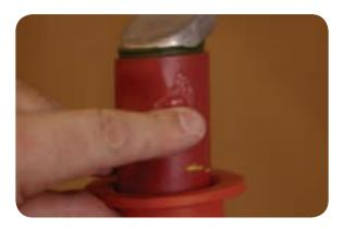
Apply a thin layer of silicone grease to the bushing.
