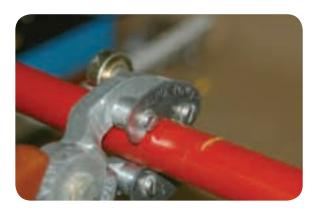
Make two longitudinal cuts (180° apart) using the PG3 sheath stripping pliers, starting 35mm beyond the circular cut and extending towards the open end of the cable.
