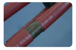
Rounding of the conductor with water pump or similar pliers assists this operation and helps prepare the conductor for insertion into the appropriate connector.
