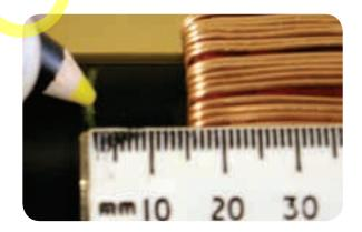
Wrap a one-third-lap layer of red sealant tape from the mark on the insulation screen up over the copper screen wires to the wire binder. Ensure that there are no gaps in the tape as this is an important moisture seal for the completed joint.
