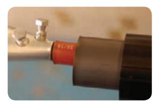
• Starting with the two bolts on the single cable end, tighten all the bolts in sequence in several steps until the heads shear off.
