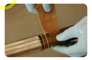
• Install five layers of PVC tape over the prepared belt and carbon papers, sticky side out, to ensure that the papers are not damaged by the next step.
