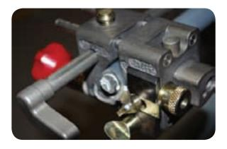
Rotate the tool along the core using the spiral cut setting until the stop gauge prevents it
