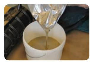
• Pour approximately half of the sand supplied in the plastic bag into the bucket and stir until it is thoroughly mixed into the resin.
