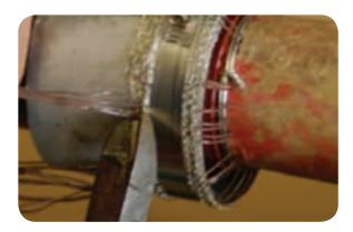
Bend the long length of 'cheese-grater' strip to form a circle and position it on the support ring, at the opposite end from where the copper wires have been fixed to the support ring.
