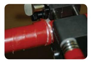
Remove the outer sheath by unwinding the spiral made by the stripping tool.
