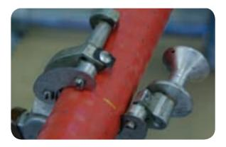
Now make a lengthwise cut along the PVC sheath between the two circular cuts.
