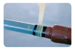
• Install the red core tubing over the cable up to the wire binder.
