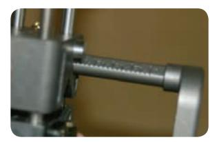
• Position the tool at the open core end. Adjust the blade to the required depth, which is just deep enough so the blade does not damage the conductor.
