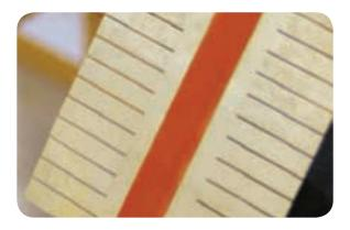
• Wrap the earth clip around the cable so that the red sealant strip is located over the red sealant on the sealing sleeve, and that the fingers of the earth strip are positioned over the copper mesh. Secure in place with a double width copper wire binder. 'Dress down' the ends of the clip to suit the size of the lead sheath.
