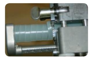
Remove the tool and the removed insulation spiral.
