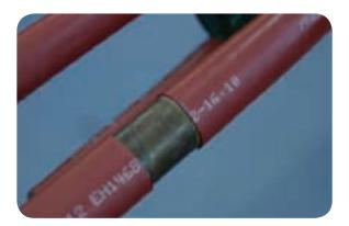
• Rounding of the conductor with water pump or similar pliers eases this operation and helps prepare the conductor for insertion into the appropriate connector.
