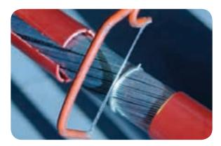
• Wear suitable gloves while removing the armour. Lift and unwrap the armour wires a few at a time and break them off against the binder by bending them backwards and forwards.
