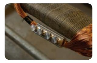
Shear off all four bolts on the mechanical connector, ensuring that the top plates do not slip out.
