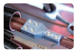
Position the three pieces of short red tube so that they butt up with the single end of the connector and shrink into position, starting from the end closest to the connector.
