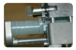
Remove the tool and the removed insulation spiral.
