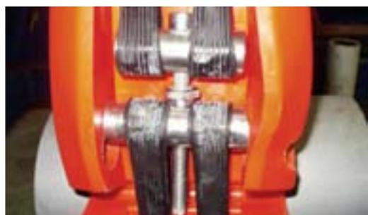
Kevlar Strap and Tensioning Assembly under Load Testing
