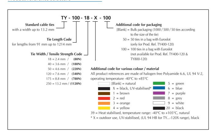
Note: Nylon (Polyamide) is inherently susceptible to environmental conditions. Ty-Fast® cable ties are moisturised to optimum performance levels at machine-side and should be stored in cool dry areas out of direct sunlight. Cable ties are packaged in plastic bags to contain moisture and should remain sealed until ready for use.
