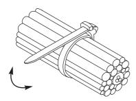
Pull end of tie through head. Turn tie end back on itself and insert into side of clip.
