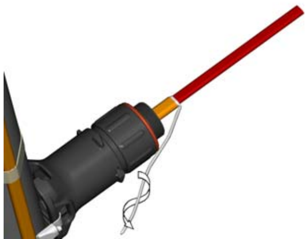
C3. Twist braid into a pigtail. Trim ends of braid.
