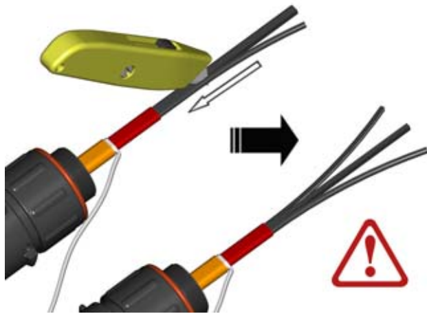
E1. Cut matrix core between inside edges of conductors. Do not cut bus wire strands.
