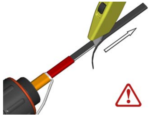
C5. Skive outside edges of black matrix. Do not cut bus wire strands. See page 19 for TSX cable matrix removal tips.
