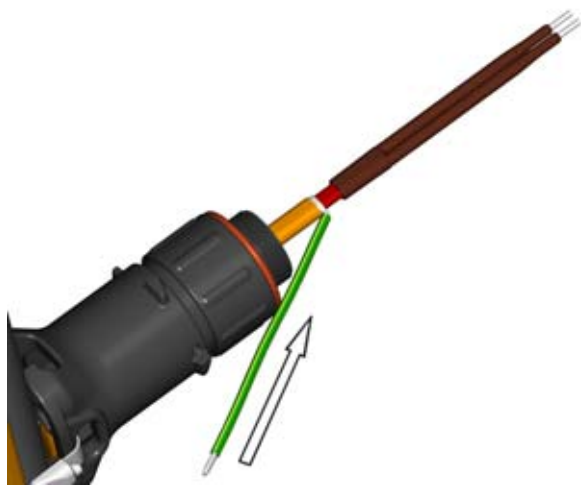
D9. Slide green/yellow ground sleeve over twisted braid.
