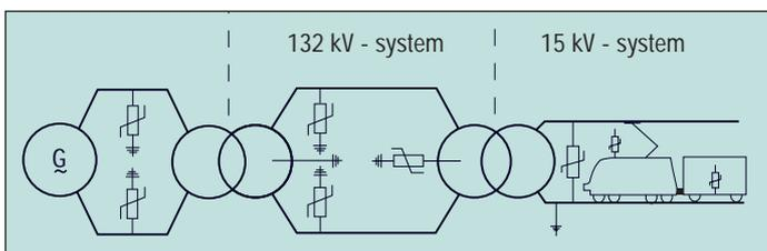
Figure 13 Schematic representation of a  $16\frac{2}{3}$  Hz railway current supply and the application of surge arresters by the Swiss National Railways.
