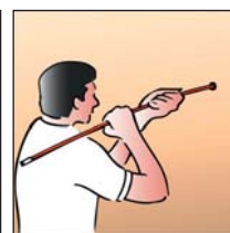
Brass Rod end being used to connect two 5mm Rods
