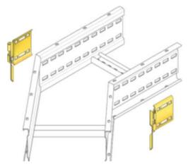
Horizontal hinged couplers shown as a pair in use to create an offset connection between two ladders
