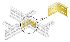
Horizontal adjustable coupler shown formed to 90° to join a ladder to a main run
