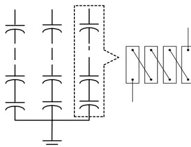
Fig 4 – Fuseless shunt capacitor bank and series string
