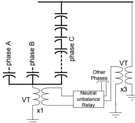
Fig. 10 – Compensated Neutral Voltage Unbalance method
