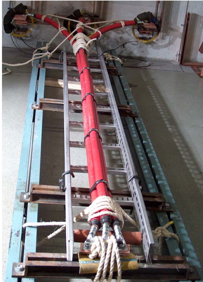
Figure 1: 300 mm 2 cable installations. Double loop cable ties with cushion sleeving mounted with a distance of 0,6 m.
