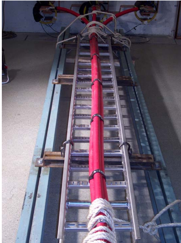
Figure 2: 300 mm 2 cable installations. Double loop cable ties with cushion sleeving mounted with a distance of 0,6 m.
