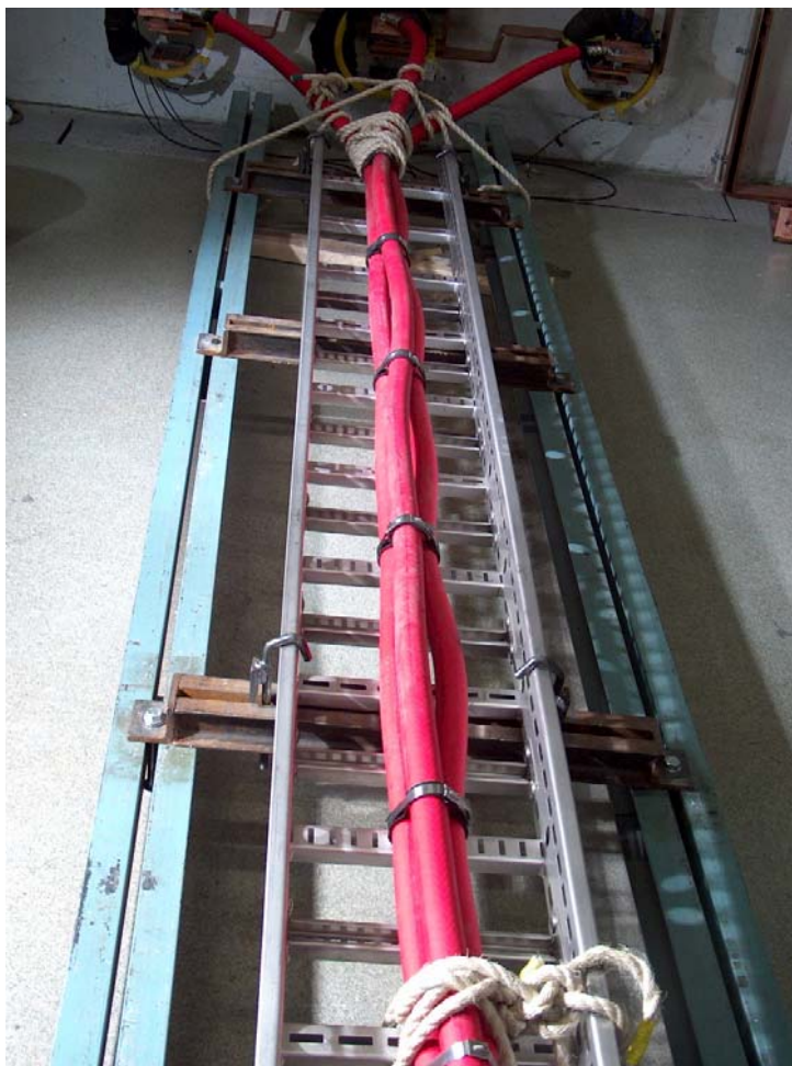
Figure 3: 240 mm 2 cable installations after one short-circuit. Single loop cable ties with cushion sleeving mounted with a distance of 0,6 m.
