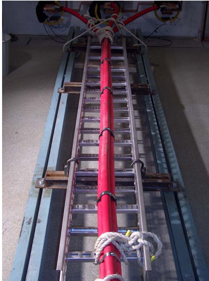
Figure 3: 240 mm 2 cable installation. Single loop cable ties with cushion sleeving mounted with a distance of 0,6 m.
