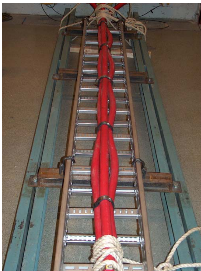
Figure 5: 300 mm 2 cable installations after one short-circuit. Double loop cable ties with cushion sleeving mounted with a distance of 0,6 m.
