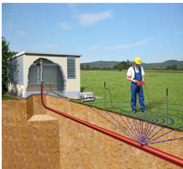
Fig. 12: Principle of the pinpointing with voltage gradients
