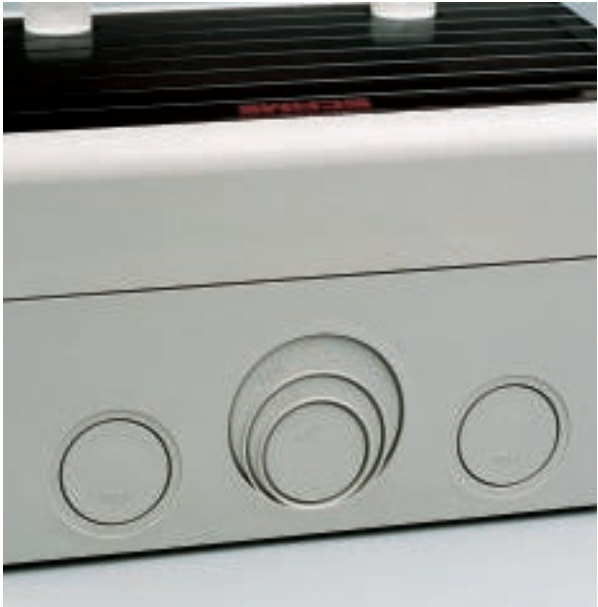
Knock-out cable entries: the required size can be knocked out using a screwdriver and hammer, making installation easier
