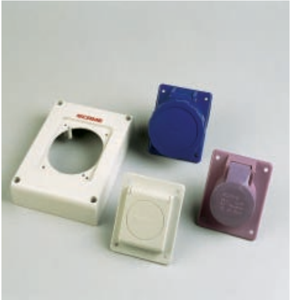
Cutouts: SCAME boxes with cutouts accept 16A IEC309 or EUREKA Series panel mounting socket outlets (70x87 mm flange) with IP44 and IP67, and socket outlets for domestic applications (section 2.2).
