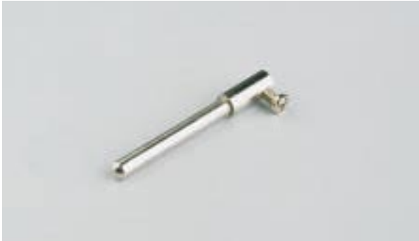
Contact pin: a component which establishes electric contact in plugs; it is manufactured from a solid brass bar and is nickel-plated to ensure it withstands corrosion and abrasion.
