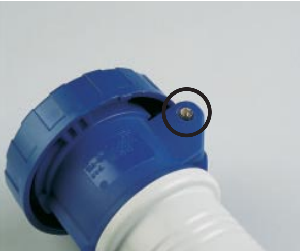
Blue: rated operating voltage between 200 and 250 V~. Slot: facilitates opening of the lid and prevents the basket from moving when closing.
