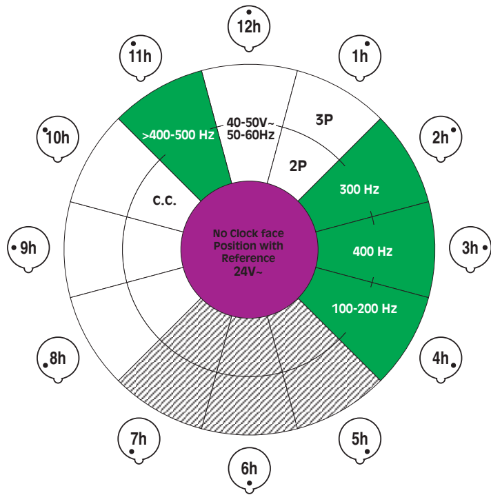
CLOCK DIAGRAM Clock face position (h) of the minor keyway of extra-low voltage (<50 V) industrial plugs and sockets to IEC 309-2 for different applications (polarity, voltage, frequency, current).
