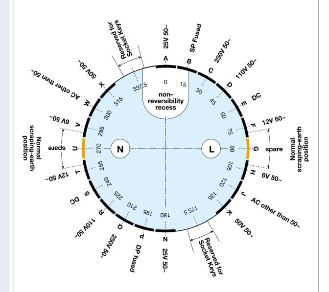
View looking at the front face of the socket-outlet or connector.
