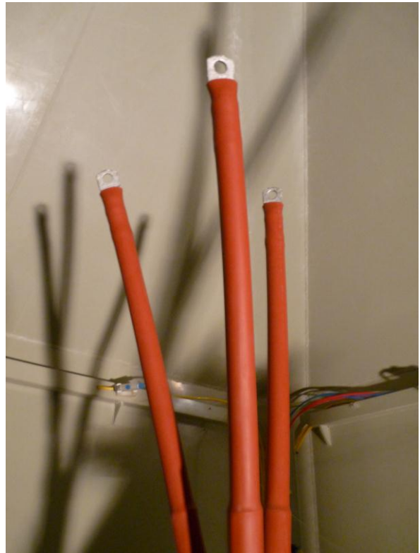
Figure 4, top of termination at 300 hours
