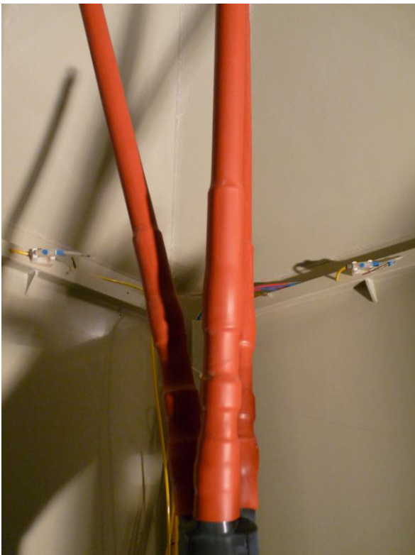
Figure 5, Bottom of termination at 300 hours
