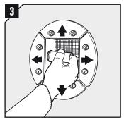
Push the front fittings to the sides. Lubricate the inside of the frame thoroughly, especially into the corners.
