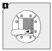
Cut or bend the net with a knife, or your fingers, to enable cables/ pipes to pass through at their position in the frame.
