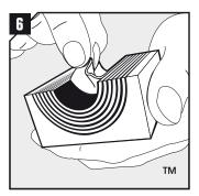
Adapt modules which are to seal cables or pipes by peeling off layers until you reach the gap seen in pic. 7. The halves may not differ by more than one layer.
