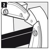
If pipes/cables are pre-routed, an R frame can be cut open with a sharp tool. Cut the longside open between screws.
