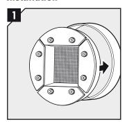
Lubricate the frame sparsely on the outside with Roxtec Lubricant. Remove any dirt and insert the frame into the sleeve/hole. Please see table "Aperture dimensions".
