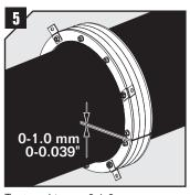
Try to achieve a 0-1.0 mm gap between the two halves when held against the cable/pipe.
