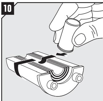
10 Lubricate thoroughly on the inside surfaces and sparsely on the outside of the seal with Roxtec Lubricant.
