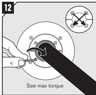
12 Tighten the screws crosswise. The seal will compress and seal the transit. Please see table for recommended max torque.
