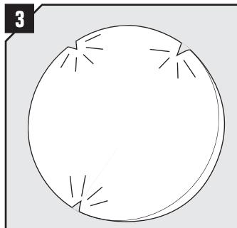
Remove all sharp edges that could damage the compression rubber.
