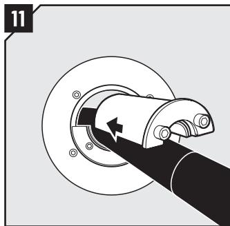
11 Insert the halves, one by one, into the sleeve.
