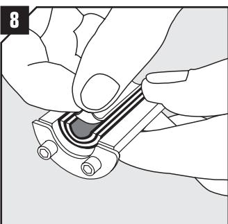
Adapt the RS seal to the cable/pipe by peeling layers from the halves until you reach the gap seen in pic.9. The halves may not differ by more than one layer.
