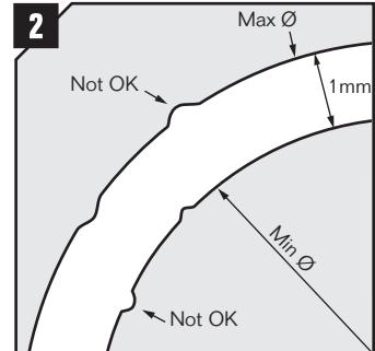
Aperture irregularities are acceptable within min and max diameters.
