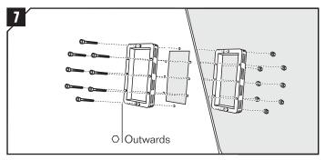
Place the frame parts with the gasket side against the wall and insert all bolts and nuts. Recessed bolt holes must point outwards, away from the wall structure.
