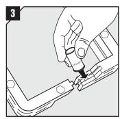
Lubricate all end surfaces of the frame parts with Roxtec Lubricant.
