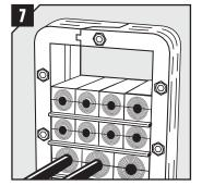
Continue to fill up the packing space of the frame, until one final row is left. See pictures "Packing space" for the full size of the space.
