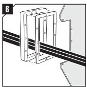
Remove the protection foil from the gasket. Apply the gasket onto one of the frame parts.
