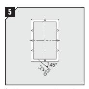
If cables are pre-routed, you will have to cut the gasket in a  $45^{\circ}$  angle, on the short side, to be able to mount it.
