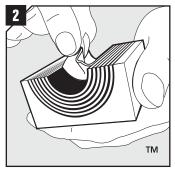
Adapt modules, which are to hold cables or pipes, by peeling off layers until you reach the gap seen in pic. 3. The halves may not differ by more than one layer.
