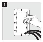
Make sure that all inside surfaces of the frame are free from dust or dirt. Lubricate the inside surfaces with Roxtec Lubricant, especially into the corners.
