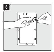
Insert and tighten all the bolts to 7 Nm.
