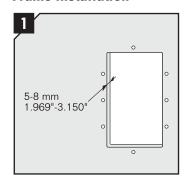
Make an opening according to aperture dimensions. The wall must be 5-8 mm thick.
