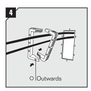
If cables are pre-routed, reconnect the frame parts around the cables. One frame part onto each side of the wall structure. Recessed bolt holes must point outwards, away from the wall structure.
