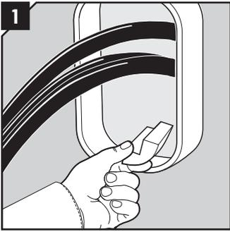
Insert the lubricated RM 40/0 RC modules in the bottom corners.
