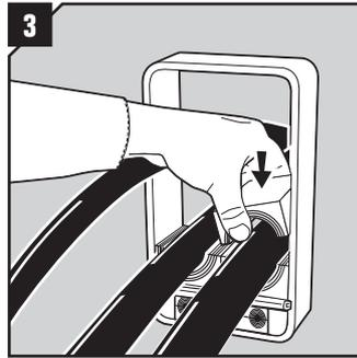
Continue to fill up the packing space of the frame according to your installation plan (transit plan). It is recommended to seal cables/pipes at the bottom of the frame and put spare modules on top.
