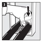
Insert the modules according to your installation plan (transit plan). It is recommended to seal cables/pipes at the bottom of the frame and put spare modules on top.
