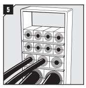
Continue to fill up the packing space of the frame, until one final row is left. See pictures "Packing space" for the full size of the space.
