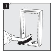
Make sure that the inside surfaces of the frame are free from dirt or dust.
