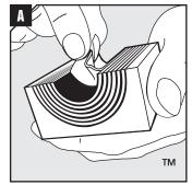
Adapt modules, which are to hold cables or pipes, by peeling off layers until you reach the gap seen in pic. B. The halves may not differ by more than one layer.
