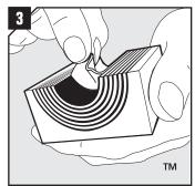
Adapt modules, which are to hold cables or pipes, by peeling off layers until you reach the gap seen in pic. 4. The halves may not differ by more than one layer.
