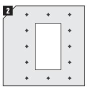
Use the frame as template for the flange hole pattern. Hole in flange  $\emptyset = 10 \text{ mm } (0.394)$ ").
