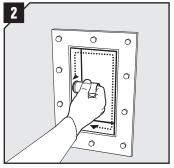
Lubricate the inside surfaces of the frame with Roxtec Lubricant, especially into the corners.
