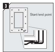
Attach the frame to the wall using bolts and nuts or other suitable fasteners. The TSL 15x6 sealing strip shall be placed between frame and wall.
