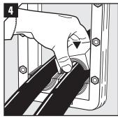
Insert the modules according to your installation plan (transit plan). Start with the largest modules.
