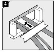
Insert all the cables and the stayplate/s into the frame.
