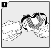
Lubricate all modules thoroughly with Roxtec Lubricant, both the inside and the outside surfaces.
