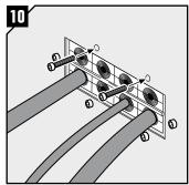
Fasten the frame to the wall with the last two screws from the backside.
