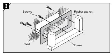
Fasten the frame loosely to the wall with four screws. The rubber gasket shall be between the frame and the wall.
