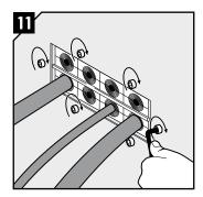
Tighten the screws on the backside diagonally.
