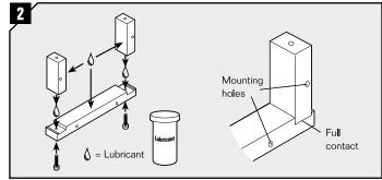
Put the two "short" frame parts and one "long" part together. Lubricate the contact surfaces. Make sure all mounting holes for the wall are on the same side and are fitted to the aperture dimensions.
