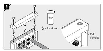
Lubricate the last "long" frame part on the inside and on both contact surfaces. Assemble the frame by tightening the screws diagonally until the "long" frame part is in full contact with the "short" frame parts.
