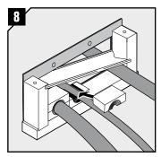
Insert the modules around the cables.
