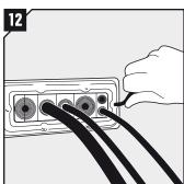
Tighten the torx screws crosswise when all modules are in place.
