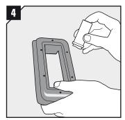
Thoroughly lubricate the compression gasket with Roxtec Lubricant.
