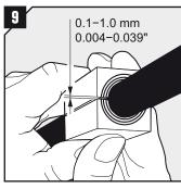
Achieve a 0.1-1.0 mm gap between the two halves when held against the cable/pipe.
