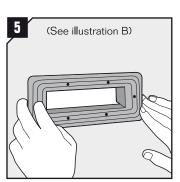
Place the compression gasket from the installation side.
