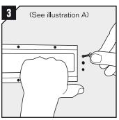
Fix the back frame with the two cross slotted screws.
