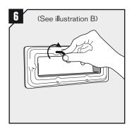
Fix the front frame parts loosely over the compression gasket with the torx screws.
