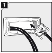
Insert the cables through the frame.
