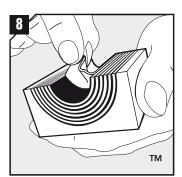
Adapt modules which are to hold cables or pipes by peeling off layers until you reach the gap seen in pic. 9. The halves may not differ by more than one layer.
