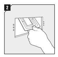
Insert the back frame from the installation side.
