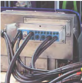
G frame in roof-top mounted equipment
