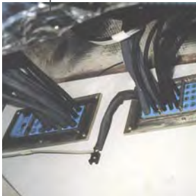
G frames in fire wall between driver's cab and passenger saloon
