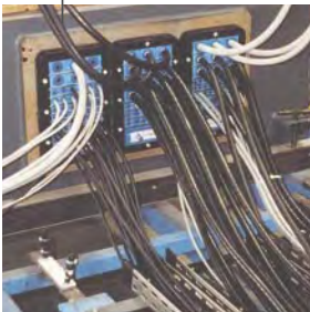
KFO frames in under-body mounted equipment
