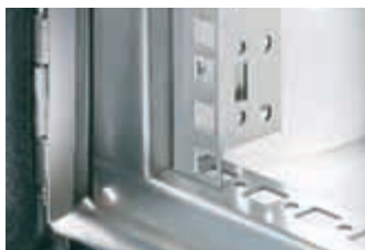
Front centre part with vertical 482.6 mm (19") mounting angle and horizontal punchings on a 25 mm pitch pattern.
