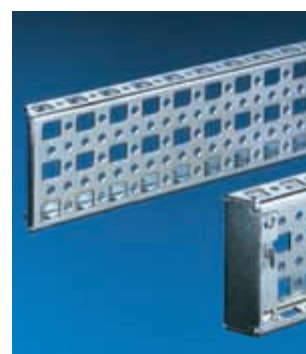
TS punched section with mounting flange 23 x 73 mm with punchings on all sides for captive nuts/threaded blocks. See Cat. 30, page 974.
