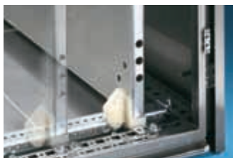
Mounting plate, zinc-plated, C fold at sides, depth-adjustable on the 25 mm pitch pattern.
