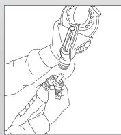
4. Remove the head by pulling the movable collar toward the base of the tool.
