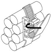
Introduce the cable tie tail into the lower slot in the head. Tighten the tie and pull it back. Slide in the tie under the catch from the side until it snaps into position.
