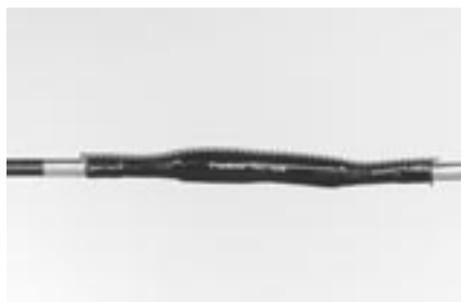
23 Wait approx. 15 minutes (cooling time) before moving the finished splice.
