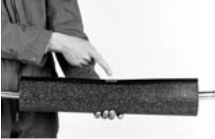
16 15 Wrap the sleeve around the splice. Press the underclip (if applicable) over the rail at the centre of the sleeve.
