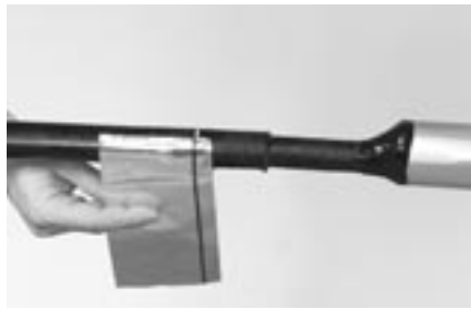
14 Apply cable aluminium foil to the cable, positioning the blue line at the mark. Smooth the foil with a blunt tool.
