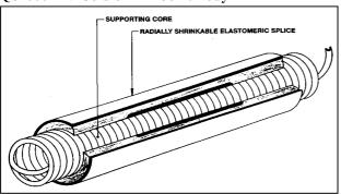
QS1000 is injection moulded and consists of three layers. A semi-conductive electrode, which forms a Faraday Cage around the connector, a high permitivity insulation layer, which both insulates and stress controls, and an outer semi-conductive layer which ensures all screens are at earth potential.
