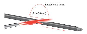
Figure A.1: Heat 2 in (50 mm) at a time
