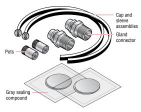
Figure 23: Termination kit with gray sealing compound
