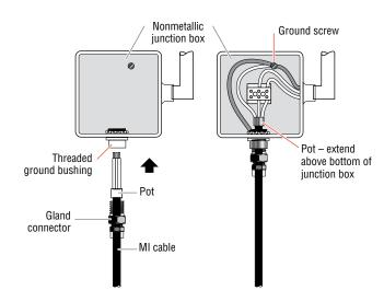
Figure 16: Connection to nonmetallic junction box
