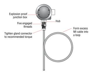
Figure 19: MI cable connection into junction box
