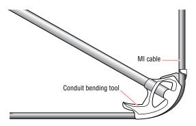
Figure 9: Use conduit bending tool for smaller bends
