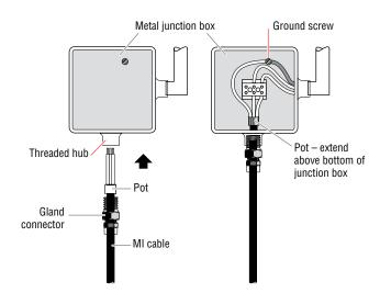
Figure 15: Connection to metal junction box
