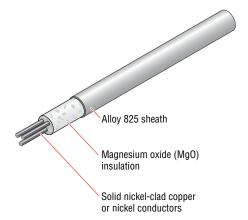
Figure 1: MI industrial wiring cable
