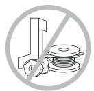
Do not lift by a single reel flange. Cable or reel may be damaged.
