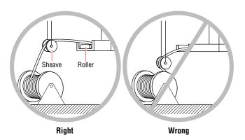
Figure 7: Reel set-up
