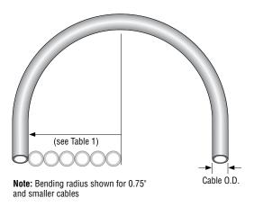
Figure 10: Minimum bending radius
