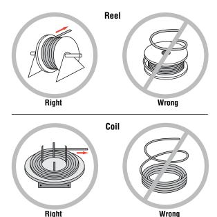
Figure 5: Unreeling/uncoiling cable
