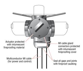
Figure 21: Fireproofing gland connectors into actuator
