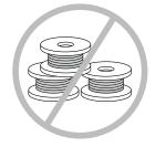
Laying heavy reels flat can cause damage.
