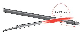
Figure A.2: Stroke flame towards end
