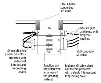
Figure 20: Fireproofing gland connectors into junction box
