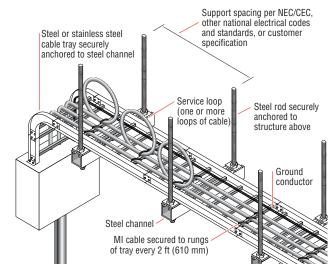
Figure 11: Typical cable tray installation using trapeze supports
