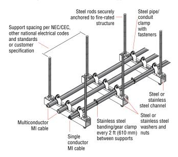
Figure 13: Typical installation using trapeze support
