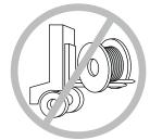
Never allow fork tines to touch the cable surface or reel wrap.
