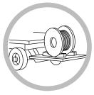
Lower reels from a truck using a hydraulic gate, hoist or fork lift. LOWER CAREFULLY.
