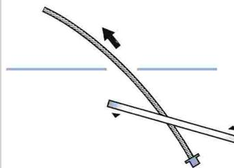
3. Ensure the toggle plate and end stop are within the cavity.
