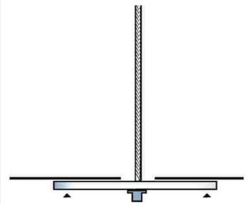
4. Pull on the wire rope to secure the plate in place.
