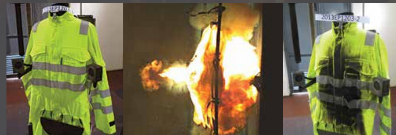
ATPV Testing. Before, during and after.
