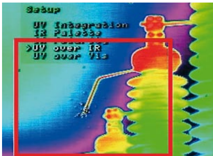
Fig. 39: Superimposed image of IR and corona measurement of the same bushing
