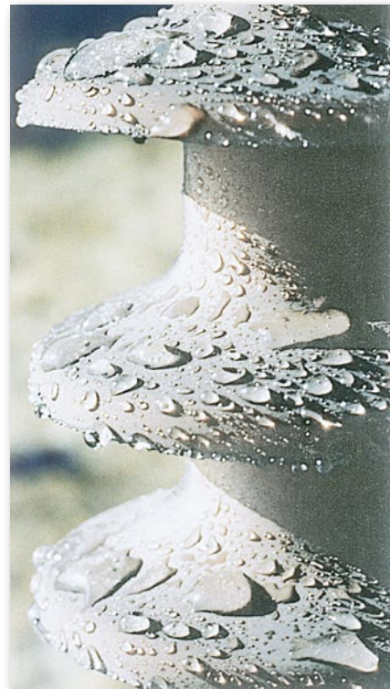
Fig. 10.2: Hydrophobicity after transfer of a polluted Silicone Rubber surface
