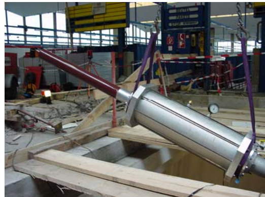
Figure 11: Test joint box with plug-in test adapter.
