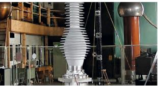
In addition to the CONNEX system, the IXOSIL ESG and IXOSIL ESU also provide conventional connections in accordance with IEC 60 859-1 for the direct introduction of XLPE-insulated cables in oil- or gas-filled equipment.
