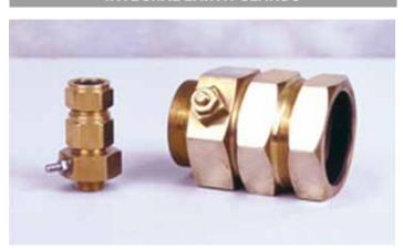
Cable Glands with an integral earth connection are recommended for use with high voltage systems. The earth connection on these glands has been successfully tested in accordance with the 43kA short-circuit test specified in BS 6121, Part 5, 1992.
