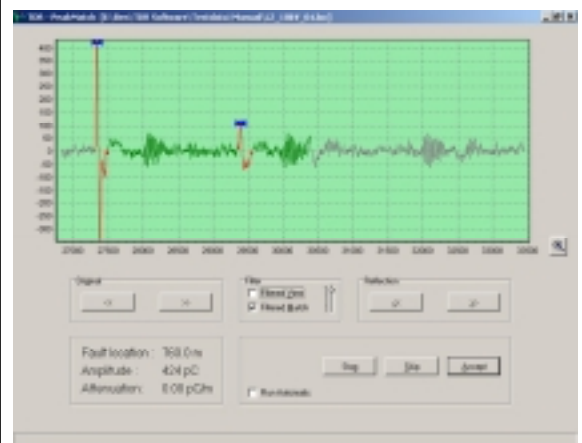
Location of PD fault positions with TDR software
