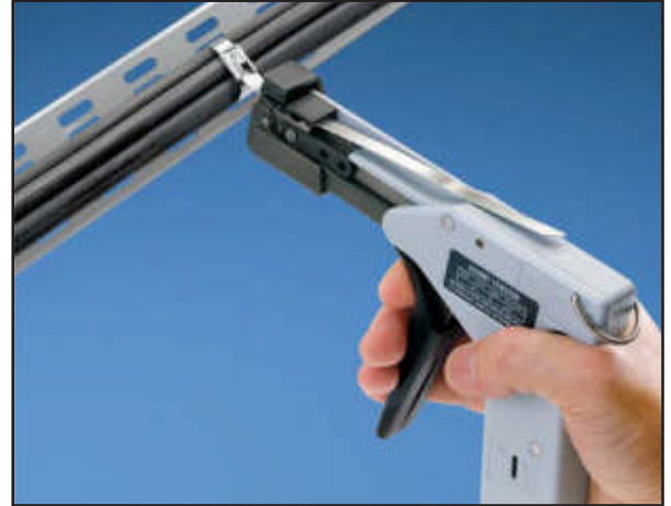
2. Use one of the PANDUIT™ PAN-STEEL™ installation tools to tension and cut off excess tail quickly.
