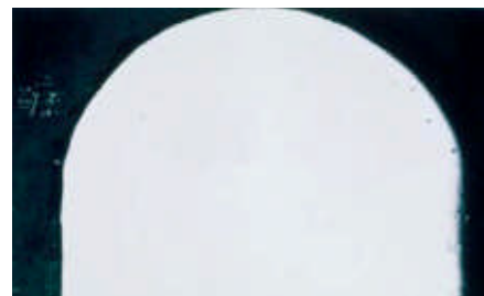
Cross sectional view of PANDUIT™ tie body. (Photo micrograph shown is magnified 150X).
