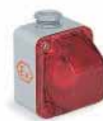
TAIS-MIGNON-Ex SERIES ATEX signal lamps in watertight wall-mounted enclosure in thermosetting material with E14 lampholder IP65
