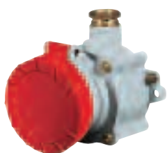
NAVE SERIES Watertight UNAV 2166 wall-mounted socket-outlets in brass enclosure painted marine grey, with UNAV 1948 cable glands 250V - IP66
