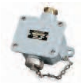
NAVE SERIES Watertight UNAV 1435 socket-outlets in brass enclosure painted marine grey, with UNAV 1948 cable glands 250V - IP66
