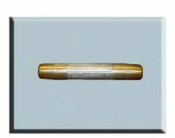
Repair sleeves are used where the strands of the conductor are broken. The sleeve is simply compressed over the damaged section of the conductor. The diameter and the length vary in order to suit the applicable conductor.
