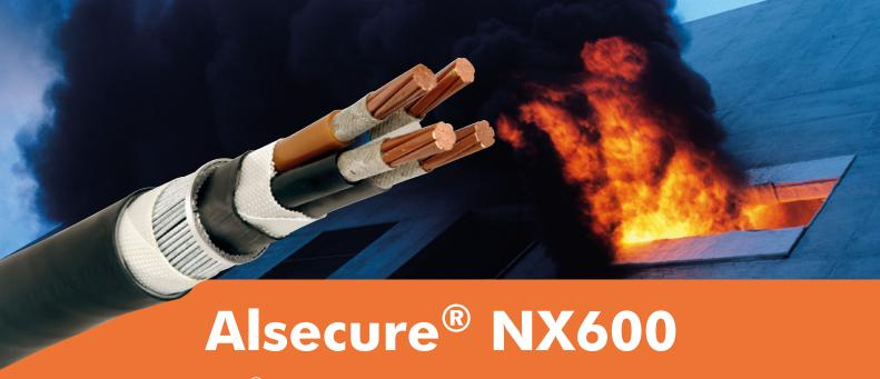
Nexans Alsecure<sup>®</sup> NX600 is a fire resistant armoured power cable that meets BS7846-F120 requirements to maintain circuit integrity in the event of a fire. It is designed for use in large, multi-storey and complex buildings such as stadia, airports, hospitals, universities, hi-rise offices and residential and public buildings.
