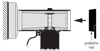
A. Installation on insulating plug BIPR without voltage detection point (for applications up to 24 kV only):
