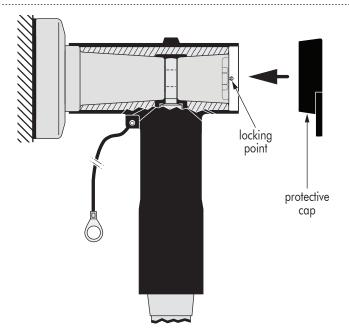
B. Installation on insulating plug BIPA with voltage detection point (for applications up to 36 kV):
