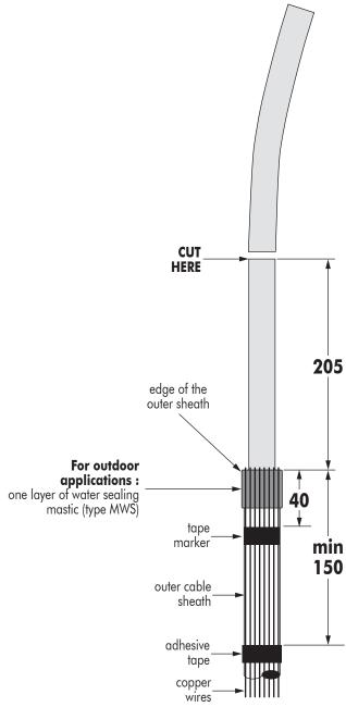
4 Apply a tape marker around the outer sheath 40 mm from the edge. For indoor applications, bend the screen wires back over the outer sheath and proceed to step no. 5.
