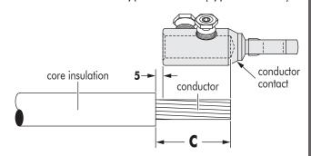
B. Remove the core insulation from the conductor for a distance « C » mm ( $\mathbf{C} = \text{depth of contact bore} + \mathbf{5} \text{ mm}$ ).
