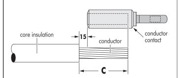
A. Remove the core insulation from the conductor for a distance **« C »** mm ( $\mathbf{C} = \text{depth of contact bore} + \mathbf{15} \text{ mm}$ ).
