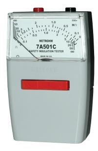
The 7A501 has been approved to BS1259 (1958) and carries the Ministry of Power Certificate Number IS1428 (Class 1) and the Factory Inspectorate Certificate Number 2148 (Class 2A and 2C) which covers Methane, Ammonia and Hydrocarbons.
